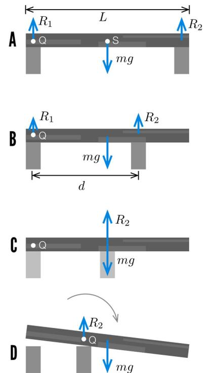
$$-R_1L/2 + R_2L/2 = 0 \implies R_1 = R_2$$
